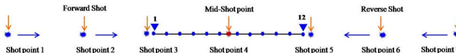
Fig. 5. A typical seismic refraction data acquisition layout and location of shot points for seismic refraction survey profile.
